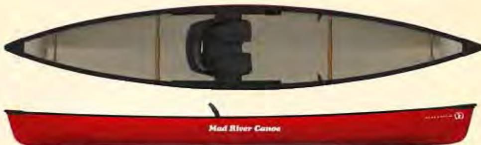
The Serenade FGX offers efficient paddling and moderate weight at a modest cost. The stiff fiberglass hybrid utilizes different fabrics to achieve the right balance of weight and durability. The hull rigidity translates into exceptional responsiveness to the paddle. Kayak-style seating is fully adjustable and conducive to use with canoe or kayak paddle.
