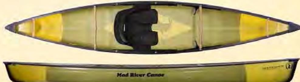
The "UL" (ultralite) aramid/core construction gives credence to an old saying - sometimes less is more. The Serenade UL is quick to accelerate, very responsive, and is extremely easy to transfer from vehicle to launch or to portage from lake to lake due to its extremely light-weight foam-core composite hull.
