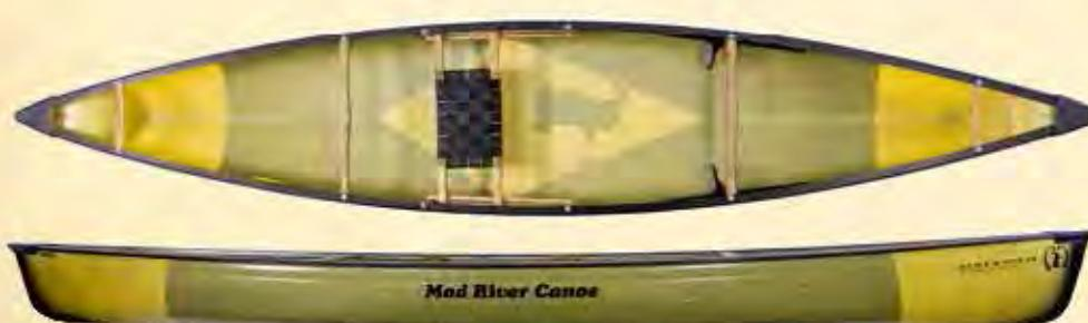
The Serenade TR Ultralite features a traditional hung sliding canoe seat for a high paddling position. Its extremely light-weight foam-core composite "ultralite" construction and simple outfitting combine to create our lightest and most efficient hull option, taking performance on the water to a new level while minimizing portage burden.
