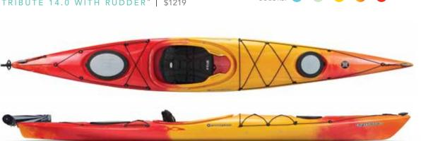
Max Capacity: 250 lbs / 113 kg Length: 14' / 427 cm Width: 23.75" / 60 cm Deck Height: 13.75" / 34 cm Boat Weight: 48 lbs / 22 kg w/ Rudder: 52 lbs / 24 kg Cockpit Length: 35" / 89 cm Cockpit Width: 19.25" / 49 cm
