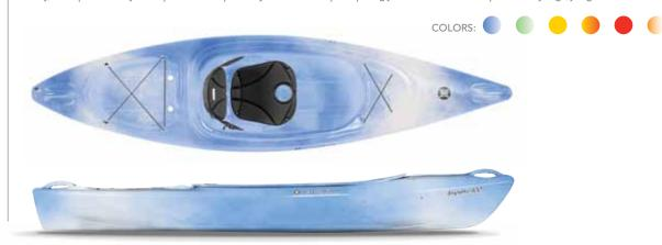
SPECS: Max Capacity: 350 lbs / 159 kg Length: 13'5" / 409 cm Width: 29.5" / 75 cm Deck Height: 15.75" / 40 cm Boat Weight: 58 lbs / 26 kg Seating Well Length: 53" / 135 cm Seating Well Width: 22" / 56 cm
