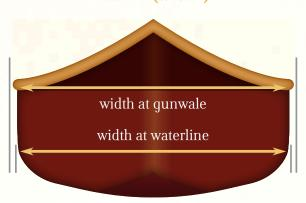
$Measured \ at the \ widest \ point \ of the \ canoe \ and \ largely \ impacts \ stability \ and \ speed. \ The \ most \ common \ reference \ is \ width \ at \ the$ gunwales but an often more telling dimension is width at the waterline as this will determine the amount of effort required to move the boat through the water.
