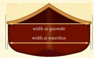
Measured at the widest point of the canoe and largely impacts stability and speed. The most common reference is width at the qunwales but an often more telling dimension is width at the waterline as this will determine the amount of effort required to move the boat through the water.
