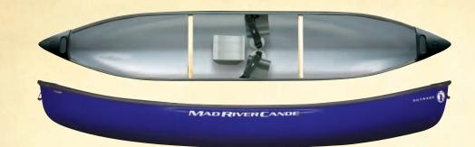
Soft chines, shallow arch hull, and extreme rocker combine to let the Outrage dance on the river. Immediate response and acceleration yield a high percentage of "made" moves for paddlers under 180 lbs. Durable Royalex construction resists and rebounds from the worst the river can throw your way.
