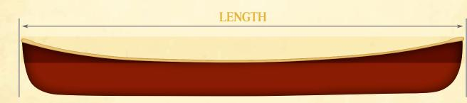
Measured stem to stem and is the most straightforward of all the aspects of canoe design. In terms of versatility, canoes in and around 16' are preferred. Large enough to be paddled tandem with a load or soloed on occasion and fast enough for touring yet nimble enough to work their way down a twisty stream. Canoes with emphasis on cruising speed tend to be longer while whitewater canoes shorter with a premium on maneuverability.
