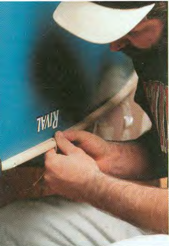
Floyd Jackson hand sands the underside of the Northern ash gunwales on a Rival. PHOTO BY ROBERT REYNOLDS
