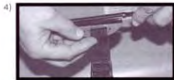
Fit wand to strap fitting
