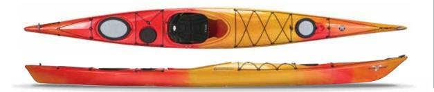
Max Capacity: 350 lbs / 159 kg Length: 17' / 518 cm Width: 23" / 58 cm Deck Height: 16.5" / 42 cm Boat Weight: 65 lbs / 30 kg Cockpit Length: 35" / 89 cm Cockpit Width: 19.5" / 49 cm
