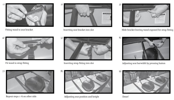
Steps  $\,$  I - 9 show you visually how to install the IQ Bucket Seat. To remove, just reverse the order of steps.
