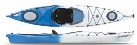
CAROLINA 12.0 The most versatile touring kayak ever created is in a category of its own. This day or weekend tripper is a performance machine, with great acceleration and speed. The soft chined and V-shaped hull offers stable, smooth paddling. The 12.0 is the perfect size to easily load and offers dry storage for gear to make the most of its capabilities.
