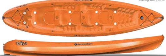
TRIBE 13.5 NEW 2010 Three's company in the Tribe 13.5 tandem. The versatile sit-on-top design features a 3-seat configuration for up to two adults and a small child or pet. Other features include self-bailing scupper tubes as well as bow and stern storage areas with bungees to safely secure gear such as backpacks, picnic baskets and coolers. Paddling solo is also no problem from the center seat.
