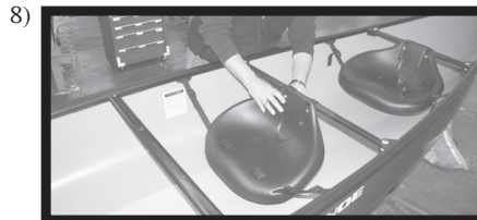
Adjusting seat position and height
