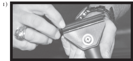
Fitting wand to seat bracket
